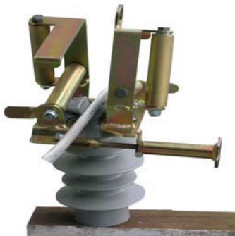
ICB-050 Still on the insulator but turned to allow the cable to drop into its tie off position.
